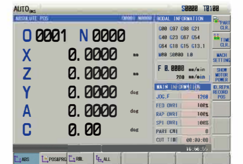
○ Record the current repair position of the thread
